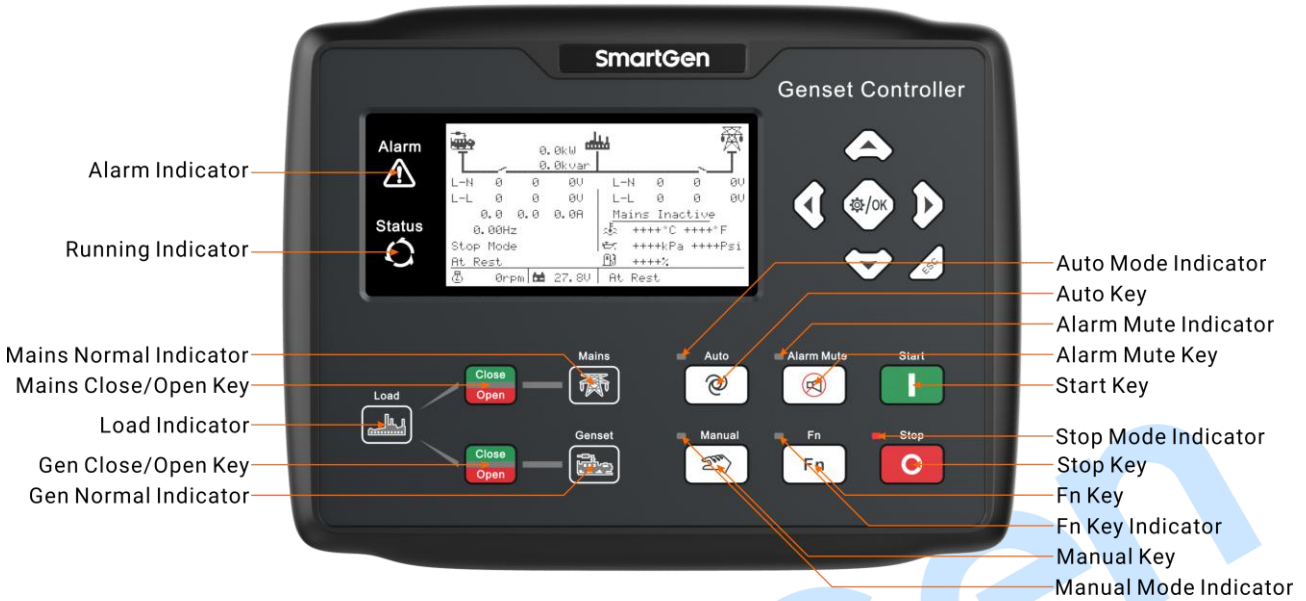
Fig.1 HGM9420N_HGM9420LT Panel Indication
